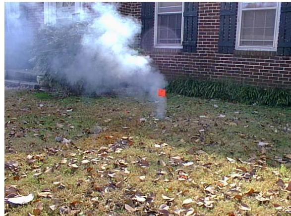
Smoke testing is the process of injecting artificially produced smoke into a blocked off pipeline segment to see where the smoke emerges. If the sewer is in good condition, then the forced smoke will emerge from manhole lids along the line and house vents on the roof. If the line has defects, the smoke will find the break and try to escape through the break.
